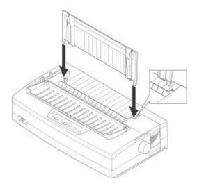
o To remove the paper guide from the printer, simply pull the tabs out of the holes.
